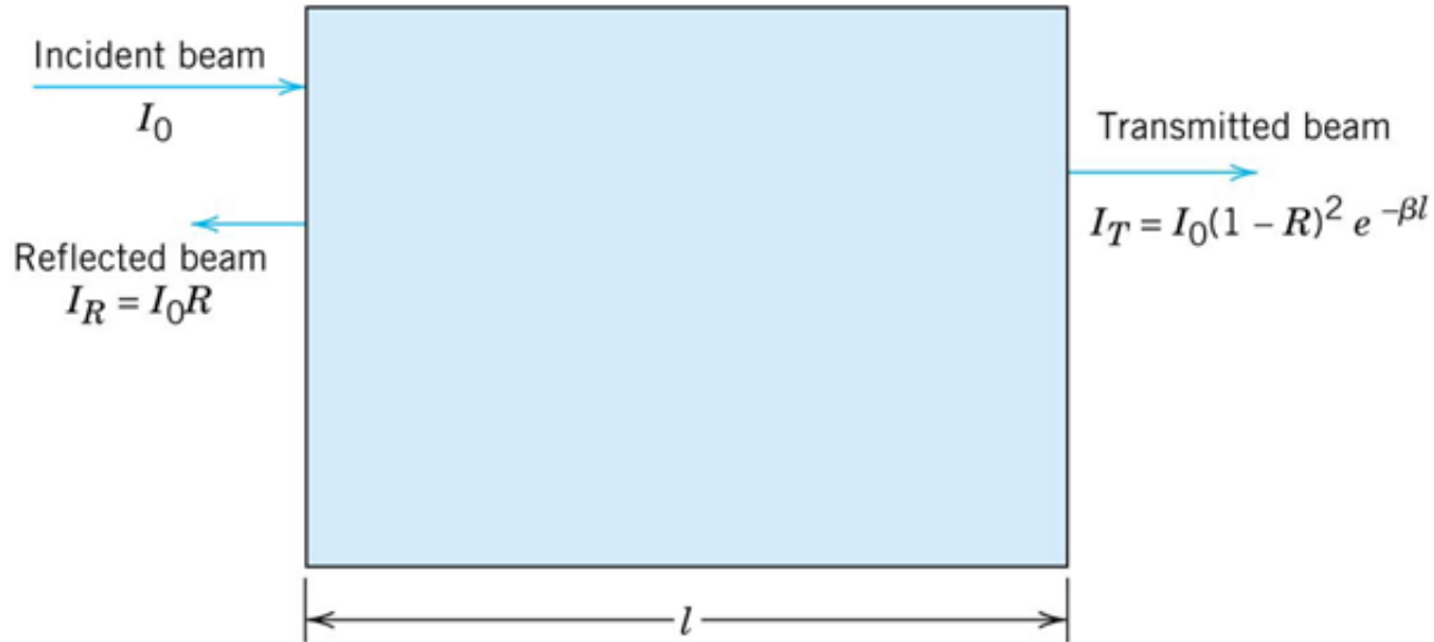
FIGURE 21.7 The transmission of light through a transparent medium for which there is reflection at front and back faces, as well as absorption within the medium.
